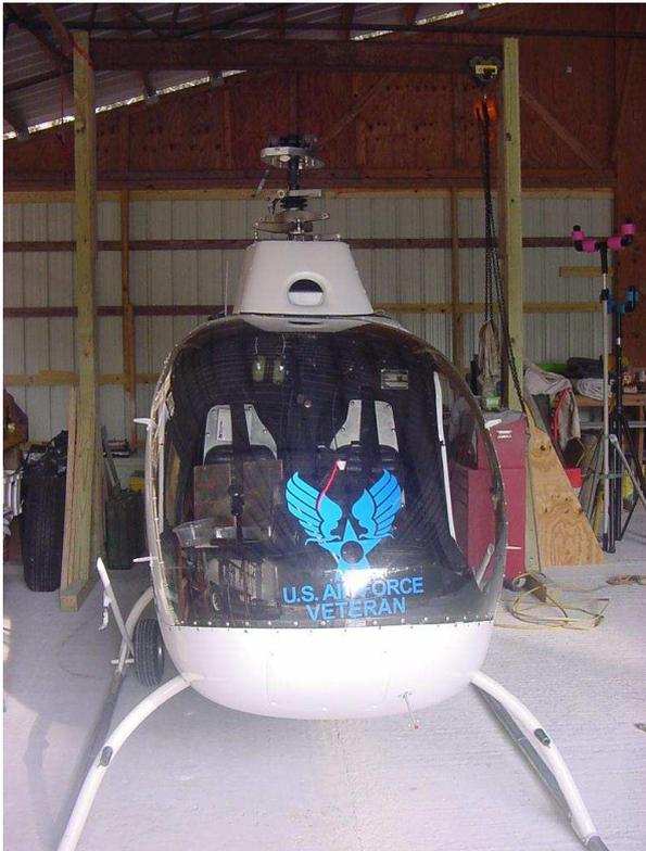
I have continued making good progress on the Rebuild of my Rotorway Exec. I have my blades assembled and painted. Still have to do the static balance and alignment on the blades. I've run the engine a few times w/o the main blades and it starts and runs well. Should be doing some testing with the blades on soon.
