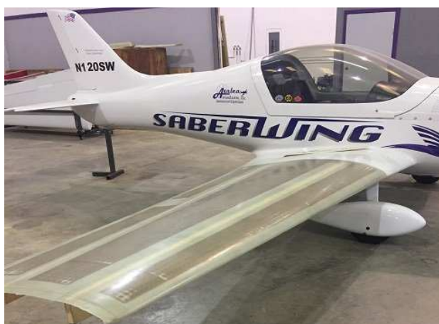
Fitting the top skin to the Prototype's spars.
